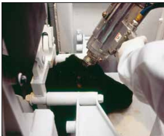
USSS-2 A Non-Penetrating Stunner with head type restrainer
