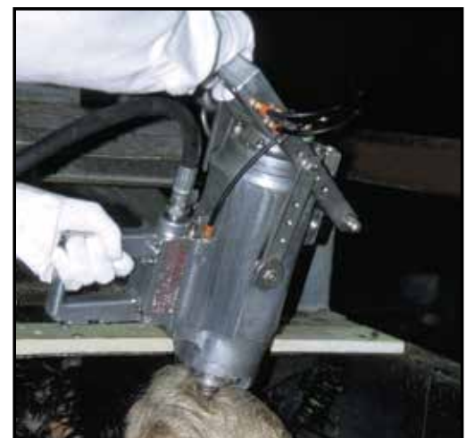
Two hand control for safer operation.
